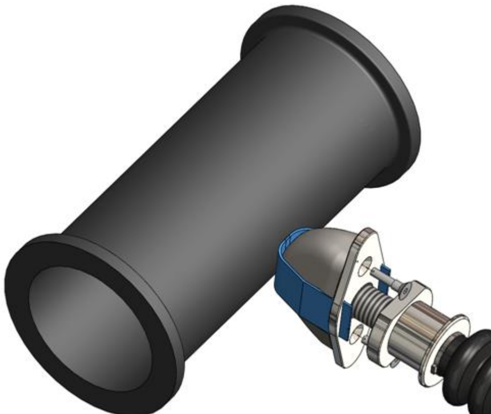
Figure 13. Installing the opening tags to pusher plate.
